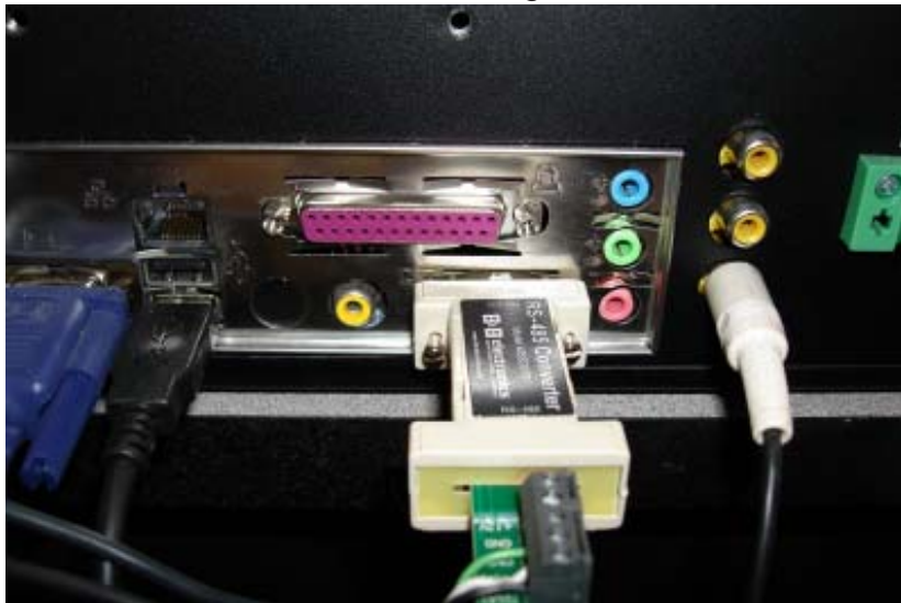
Rear panel with RS232-485 converter, USB, VGA, and video input connectors shown
