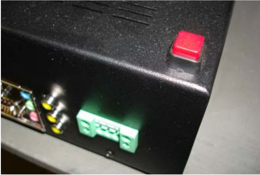
Rear panel showing power input connector and power on switch
